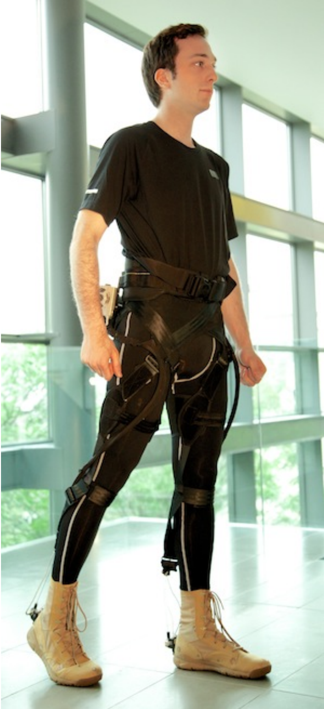
The Warrior Web Suit equipped with flexible cables and small motors. Photo: DARPA
